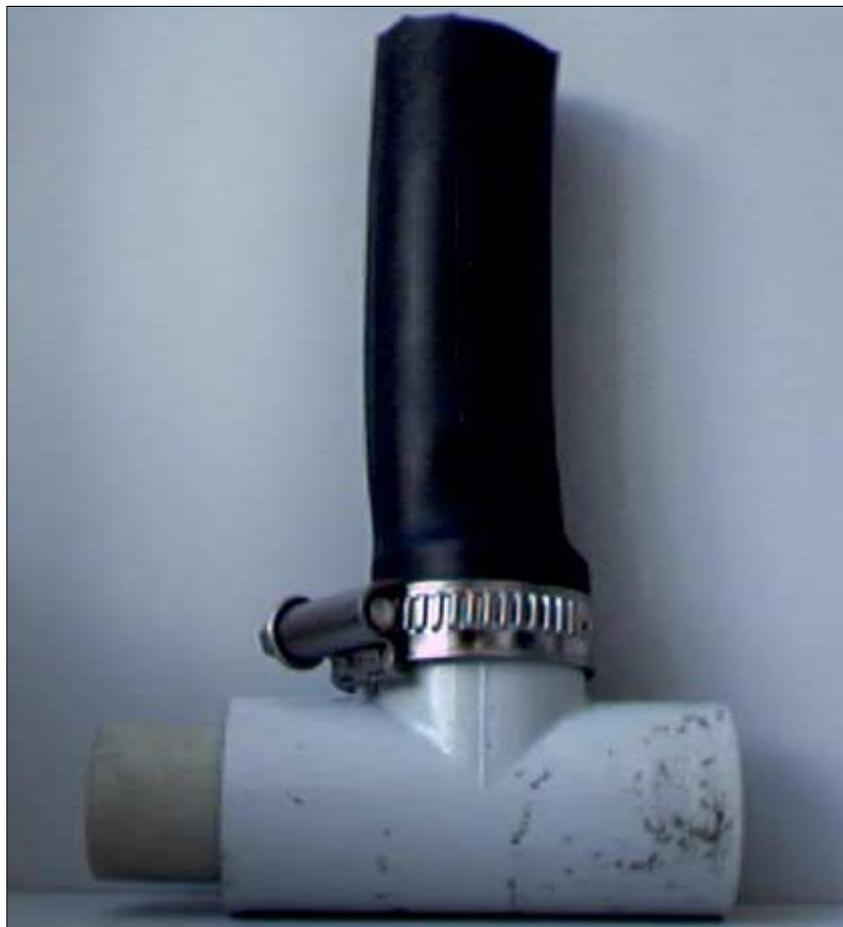
We then conducted several tests on the eductor at different pressures and with one or two air inlets. The Best result achieved was it took ten seconds for 500 grams to be moved to the top hopper.
