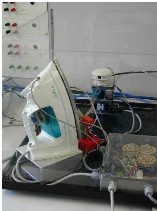
Figure 3a, 3b – Domestic electric iron used for remote laboratory exercises
